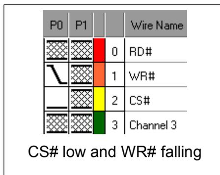
The second illustration shows the setup when we want to trigger on WR# falling edge if and only if CS# is low. In other words, *WR# falling* and *CS# low* and other wires *don't care*.
