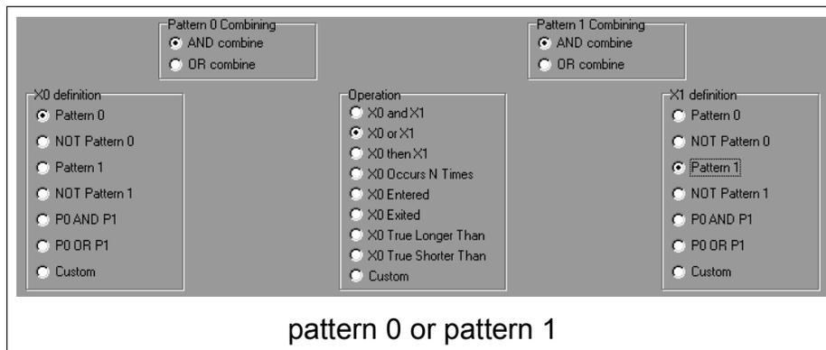
We select AND combining for both patterns, then select X0=a hit on pattern 0 and X1=a hit on pattern 1. Finally selecting the trigger as (X0 or X1) gets us what we want. Of course, there are a number of other choices we could have made to end up with the same triggering condition.
