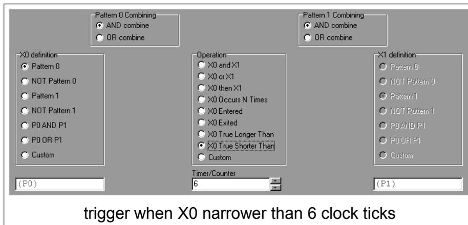
In this case we calculate the counter/timer value by dividing the clock speed. For instance, 60ns with a 100MHz (10ns) clock, gives a counter value of 6.
